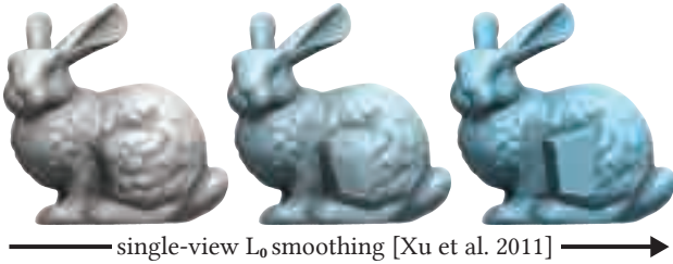
Fig. 3. The Bunny is optimized so the gradient of its rendered image for a single view is minimal in an L_0 sense.
