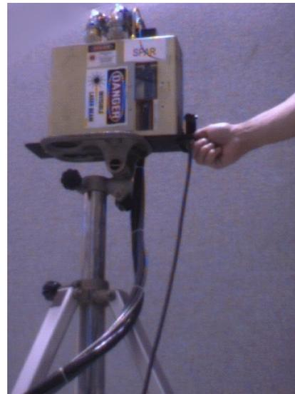
Figure 22: The SPAR laser range scanner
