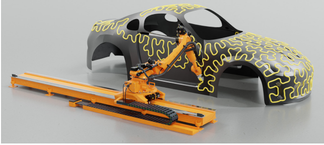
Fig. 3. Surface-filling curves can potentially be used in applications like robotic path planning for tasks including painting or polishing surfaces.
