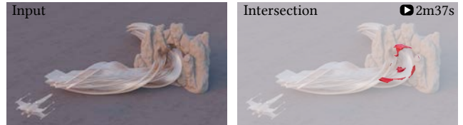
Fig. 19. The intersection between the path of a spaceship and a rock formation is computed without necessary computing the swept volume of the entire path, cutting runtime by a factor of 20. Model by Karl, CC BY-SA 3.0.
