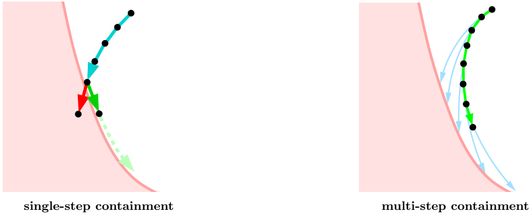
Figure 5.4: Trajectory comparison between single-step and multi-step containment. Multi-step containment tends to produce earlier and softer compliance with the viability envelope constraint.
