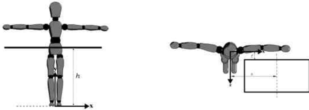
Figure 3.7 Table model dimensions (Height = h , Front = f , Skew = s ).
