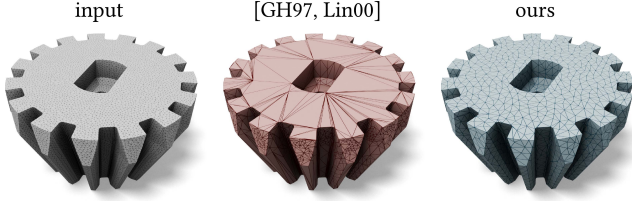
Figure 3: Although using a robust numerical solver (e.g. [LT98]) can resolve the numerical issue from the quadric error simplification [GH97], it does not change the decimation priority, leading to random edge collapses in planar regions and low-quality triangulations (middle). Sprinkling a little bit of our line quadrics ( w_i = 10^{-4} ) not only resolves the numerical issue, it further encourages uniform decimation within planar regions (right).
