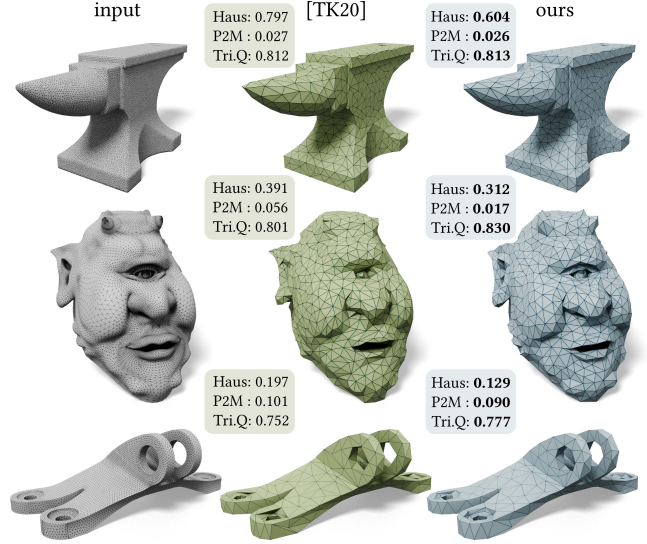
Figure 10: Compared to the probabilistic quadrics [TK20], we demonstrate that our method leads to better results by showing that our method contains Pareto optimal solutions measured by the Hausdorff distance (Haus), average point-to-mesh distance (P2M), and the triangle quality (Tri.Q).
